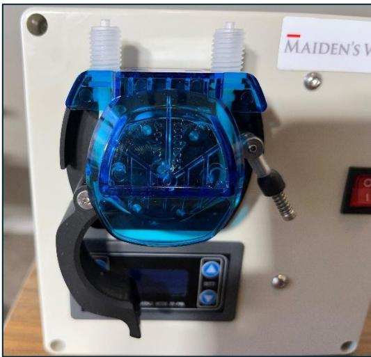
3. Undo the two screws on the top of the pump and remove the front face
