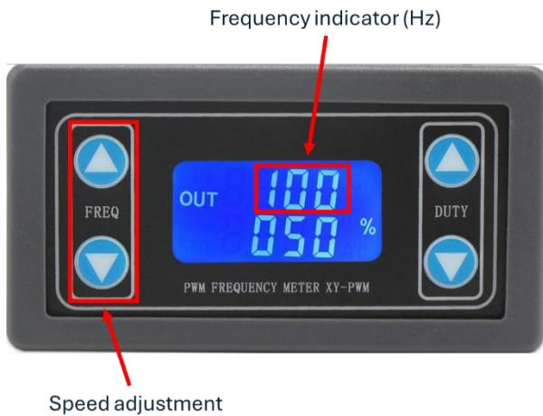
A frequency of 37.3kHz delivers the maximum pump speed of 350rpm.
