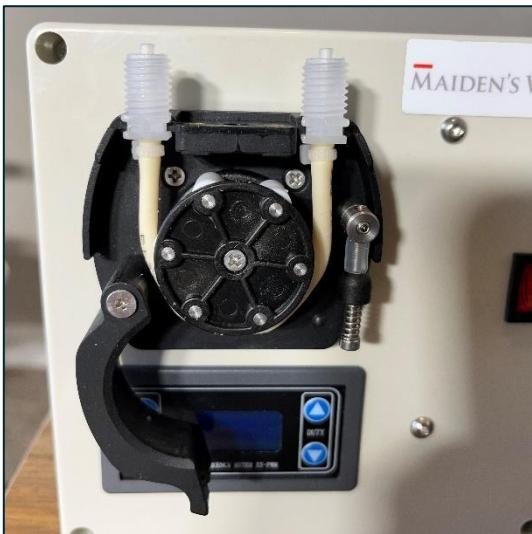
4. Slide the two threaded tube attachments out of their slots in the pump body and remove the internal tube.
