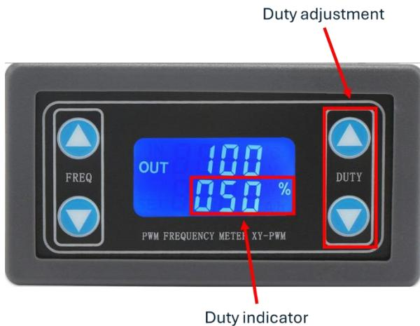
The signal frequency, and therefore pump speed and flow rate, is adjusted using the arrows as shown below.
